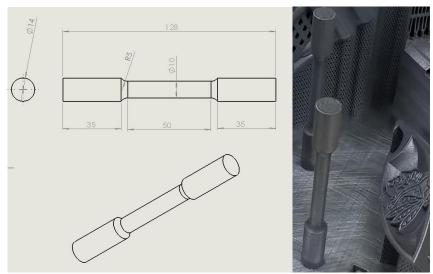
Fig.1 Tensile test bar and 3D-printing orientation
