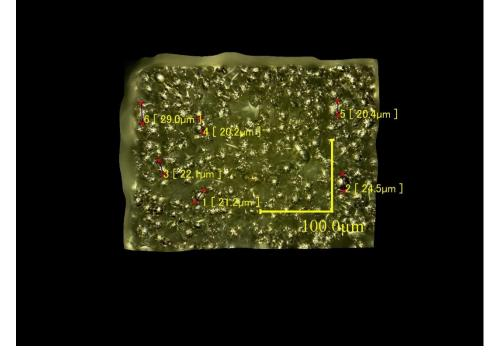
Fig.4 powder particles in microscopic image
