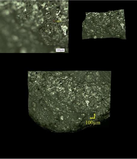
**Fig. 3** Microscopic image of the tensile test bar (upper left closer image in fracture plane, upper right is 3D image in fracture plane and lowest is bigger area image)
