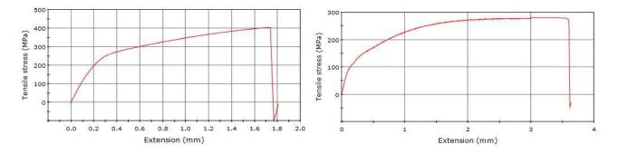
Fig.6 Tensile test graph for AlSi10Mg; without heat treatments on the left and on the right side is heat treated
